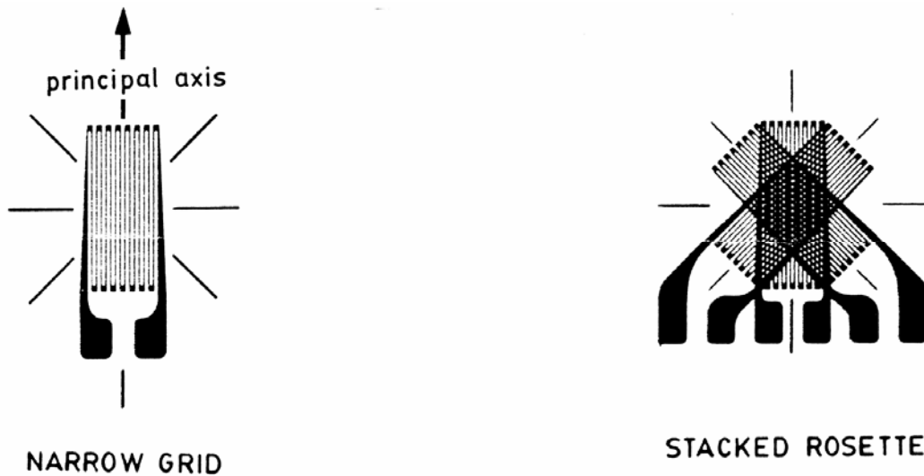
Figure 3: Foil strain gage configuration
